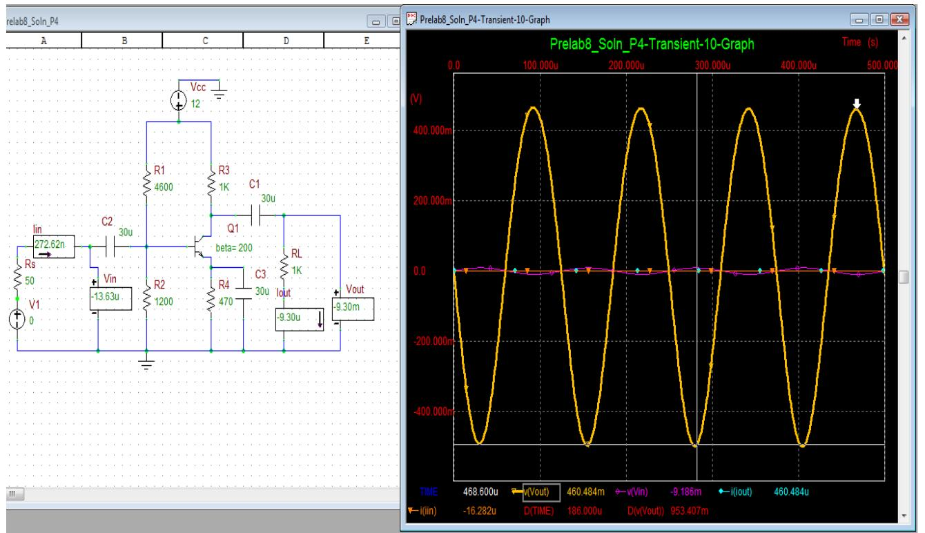
Without  $R_E = R_4$  in the circuit:
