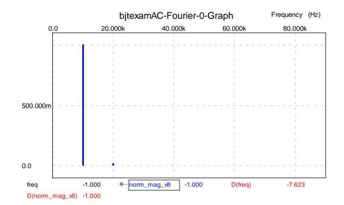
Graphic output for .08 V sine wave input (IVM1) at 10 kHz. Output is show for meter IVM2.
