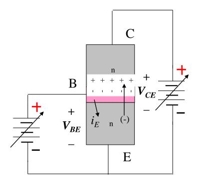
The *pn* junction for  $V_{BE}$  is forward biased and current  $i_{BE}$  flows according to the Shockley equation:
