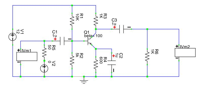
Graphic output for .03 V sine wave input (IVM1) at 10 kHz. Output is shown for meter IVM2.
