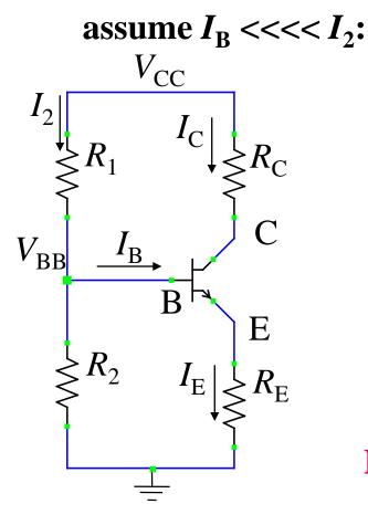
$$V_{BB} = V_{CC} \frac{R_2}{R_1 + R_2}$$
