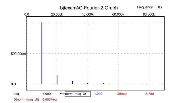
Graphic output for 1.2 V sine wave input (IVM1) at 10 kHz. Output is show for meter IVM2.
