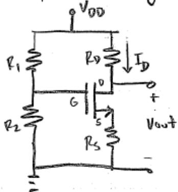
$$V_{DD} = I_D R_D + V_{DS} + I_D R_S$$
