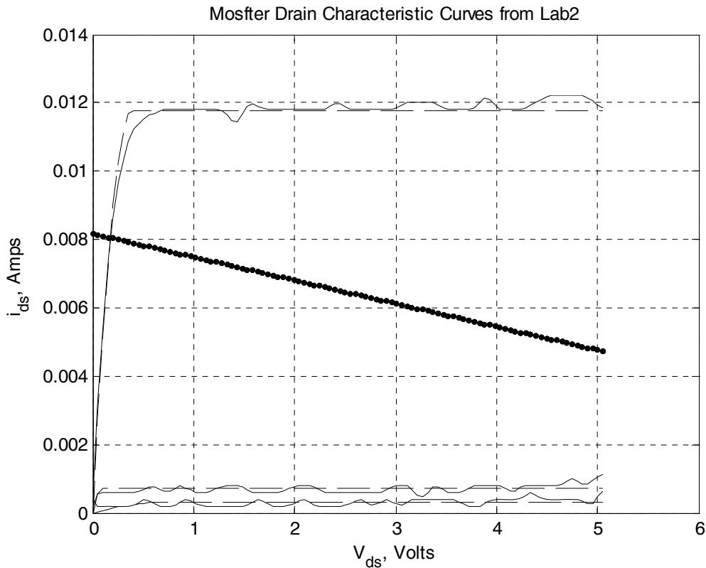
Any attempt at guessing the  $V_{GS}$  necessary to produce the quiescent point will be accepted here, as it is fairly difficult to have recorded enough of a sweep using the curve tracer previously that would allow you to accurately guess this number. The important thing here is to note where the load line crosses
