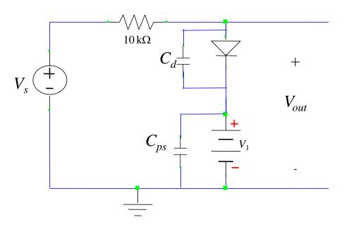
Compute effective capacitance over  $V_{out}$
