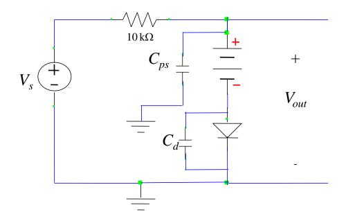
Compute effective capacitance over  $V_{out}$
