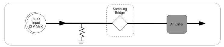
Figure 20. The architecture of a digital sampling oscilloscope.
