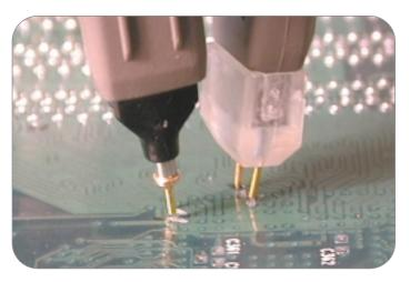
Figure 40. Dense devices and systems require small form factor probes.
