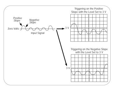
Figure 36. Positive and negative slope triggering.
