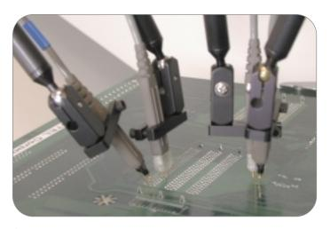
Figure 42. High-performance probes are critical when measuring the fast clocks and edges found in today's computer buses and data transmission lines.
