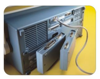
Figure 55. A TDS3000 Series oscilloscope provides a wide array of communications interfaces, such as a standard Centronics port and optional Ethernet/RS-232, GPIB/RS-232, and VGA/RS-232 modules.
