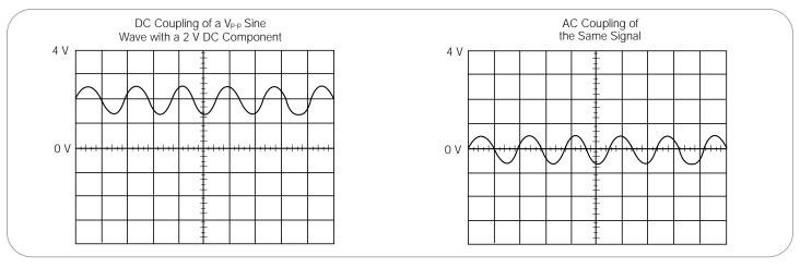
Figure 23. AC and DC input coupling.
