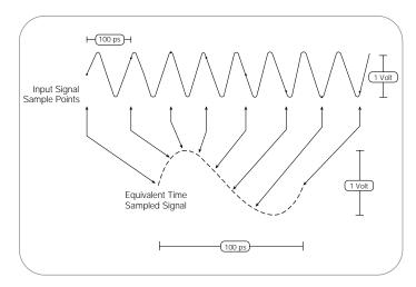
Figure 28. Basic Sampling. Sampled points are connected by interpolation to produce a continuous waveform.
