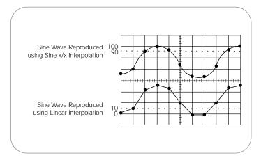
Figure 31. Linear and sin x/x interpolation.
