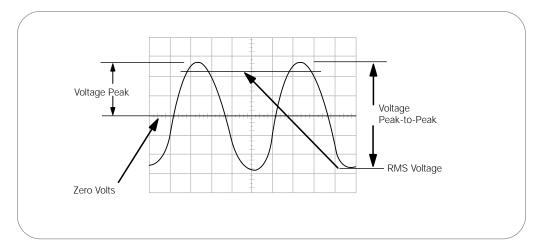
Figure 66. Voltage peak (V<sub>ρ</sub>) and peak-to-peak voltage (V<sub>ρ-ρ</sub>).
