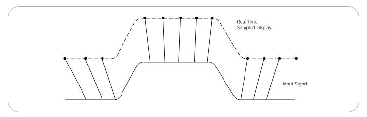
Figure 30. In order to capture this 10 ns pulse in real-time, the sample rate must be high enough to accurately define the edges.
