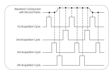
Figure 32. Some oscilloscopes use equivalent-time sampling to capture and display very fast, repetitive signals.
