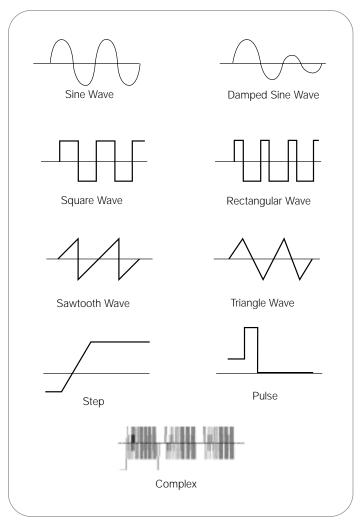
Figure 3. Common waveforms.
