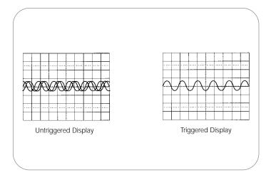
Figure 14. The trigger stabilizes a repetitive waveform, creating a clear picture of the signal.
