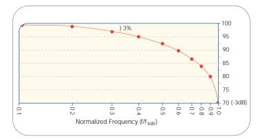
Figure 46. Oscilloscope bandwidth is the frequency at which a sinusoidal input signal is attenuated to 70.7% of the signal's true amplitude, known as the -3 dB point.
