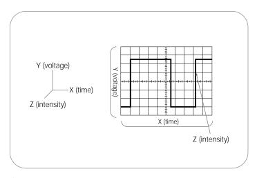
Figure 2. X, Y, and Z components of a displayed waveform.
