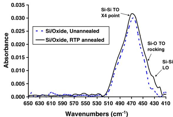
Fig. 3. FTIR spectra of thick-oxide samples (80 nm): Si/SiO<sub>2</sub> samples based on n<sup>+</sup> wafers ( $n = 1 \times 10^{19} \text{ cm}^{-3}$  and  $\rho = 5 \times 10^{-3} \Omega \text{ cm}$ ) without any annealing and with RTP annealing (1050 °C in nitrogen for 4 min).
