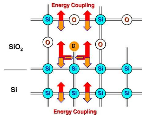
Fig. 6. Schematic illustration of phonon energy from the Si–O rocking mode coupled back to the Si–D bending mode and the Si–Si TO phonon mode.
