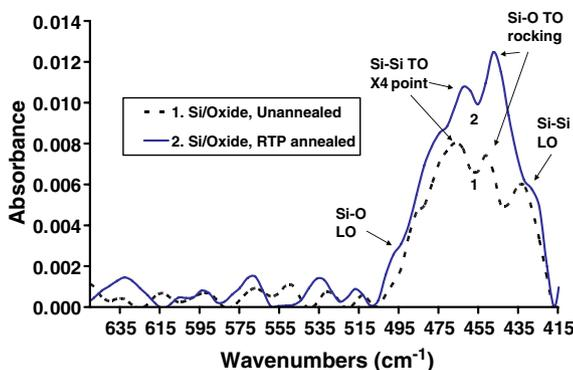
Fig. 2. FTIR spectra of Si/SiO<sub>2</sub> wafers based on n<sup>-</sup> wafers ( $n = 2 \times 10^{14} \text{ cm}^{-3}$  and  $\rho = 20.8 \Omega \text{ cm}$ ): (1) without any annealing and (2) with RTP annealing (1050 °C in nitrogen for 2 min). The oxide thickness is 29 nm.
