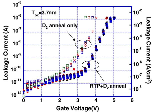
Fig. 10. Gate leakage currents of silicon MOS capacitors with oxide thickness of 3.7 nm and area of  $4.24 \times 10^{-4}$  (cm<sup>2</sup>) with D<sub>2</sub> anneal only and with RTP (1050 °C in nitrogen for 4 min) plus deuterium anneal (450 °C for 30 min).
