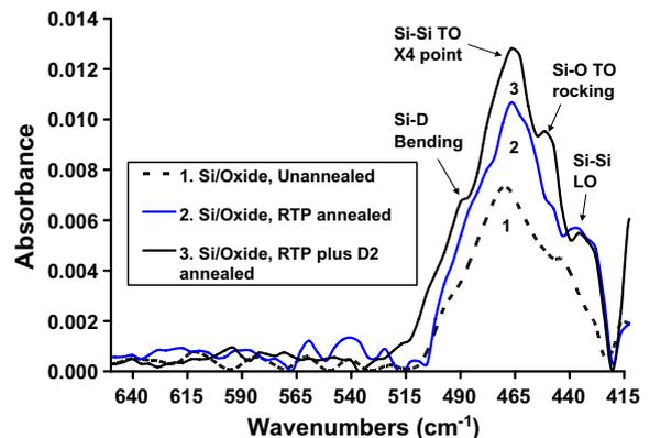
Fig. 1. FTIR spectra of  $\text{Si}/\text{SiO}_2$  samples (23 nm oxide) based on  $n^+$  wafers ( $n = 1 \times 10^{19}\text{ cm}^{-3}$  and  $\rho = 5 \times 10^{-3}\text{ }\Omega\text{ cm}$ ): (1) without any annealing, (2) with RTP annealing ( $1050\text{ }^\circ\text{C}$  in nitrogen for 4 min), and (3) with RTP ( $1050\text{ }^\circ\text{C}$  in nitrogen for 4 min) plus deuterium annealing ( $450\text{ }^\circ\text{C}$  for 30 min).
