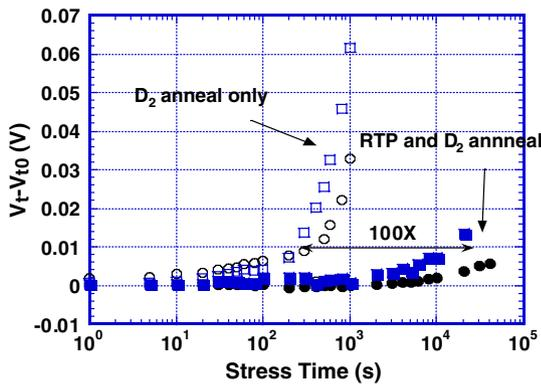
Fig. 4. Comparison of the threshold voltage shift of a MOS transistor processed in deuterium only with that processed in RTP plus deuterium anneal. The devices ( $L = 2 \mu\text{m}$ ,  $W = 150 \mu\text{m}$ , and  $T_{\text{ox}} \approx 20 \text{ nm}$ ) were stressed at  $V_G = 5 \text{ V}$  and  $V_D = 12 \text{ V}$ .
