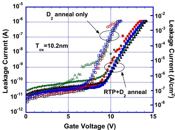
Fig. 9. Gate leakage currents of silicon MOS capacitors with oxide thickness of 10.2 nm and area of  $4.24 \times 10^{-4}$  (cm<sup>2</sup>) with D<sub>2</sub> anneal only and with RTP (1050 °C in nitrogen for 4 min) plus deuterium anneal (450 °C for 30 min).
