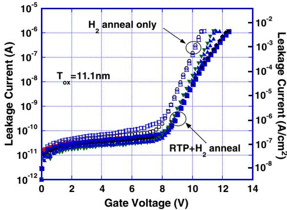
Fig. 8. Gate leakage currents of silicon MOS capacitors with oxide thickness of 11.1 nm and area of  $4.24 \times 10^{-4}$  (cm<sup>2</sup>) with hydrogen anneal (450 °C for 30 min) and with RTP (1050 °C in nitrogen for 4 min) plus hydrogen anneal (450 °C for 30 min).
