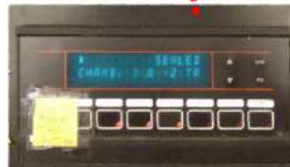
Figure 2a: Chamber pressure controller
