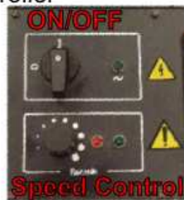
Figure 2b: Rotary workholder controller
