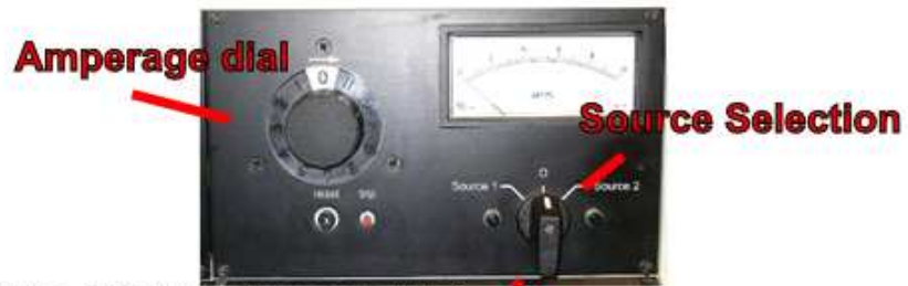
Figure 2d: Amperage control
