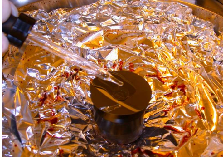
Figure 4a: Applying the coating solution
