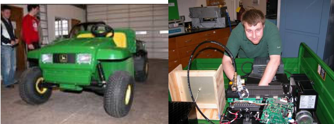
Figure 3. John Deere e-Gator with fuel cell power unit as the payload.
