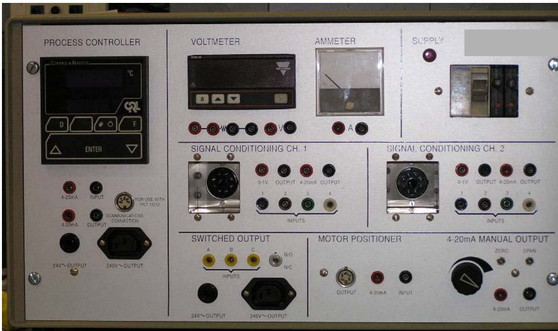
Figure 2. Control panel for pressure regulation apparatus
