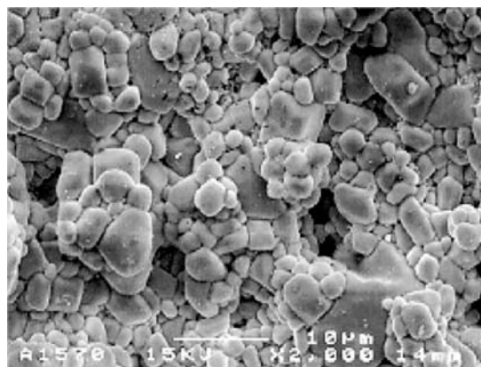
Fig. 12. Ba 1-x Sr x TiO 3 sintered at 1050 °C. Reprinted with permission from [86], W. Qu et al., Measurement Sci. Technol. 11, 1111 (2000). © 2000, Institute of Physics.
